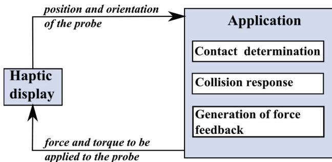
**Fig. 2.** Haptic rendering pipeline for the impedance control scheme
